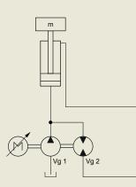
4-quadrant displacement control with hydraulic and electric energy recovery
